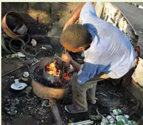
Melting the aluminium waste
